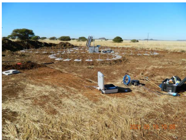
IS47 in Boshoff: New vault mounted on a cement bed and Wind Noise Reduction System.
