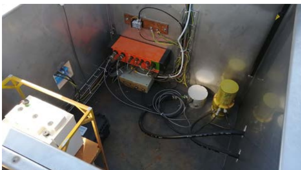
New vault at element 8 with the new Hyperion sensor connected to the wind noise reduction system and the old MB2000 sensor as a reference sensor
