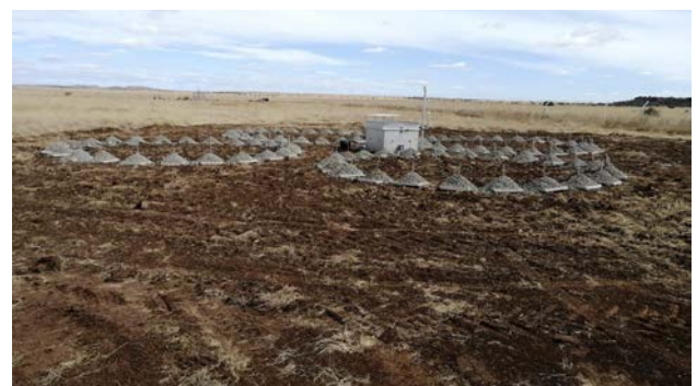
Element 1 with meteorological station installed and operational and pipe array ends covered
